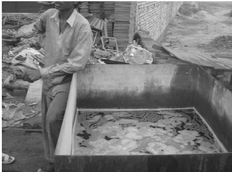
A bath for extracting copper from printed circuit board in informal recycling workshop in India. Provided by IRG Systems South Asia
