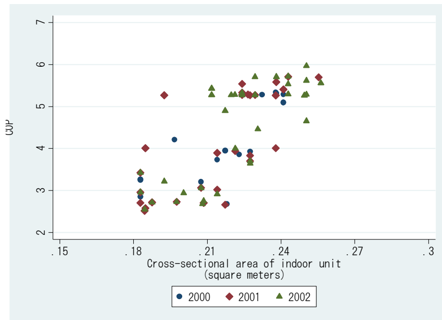
Figure 3. COP and Indoor Unit Size During 2000-2002
