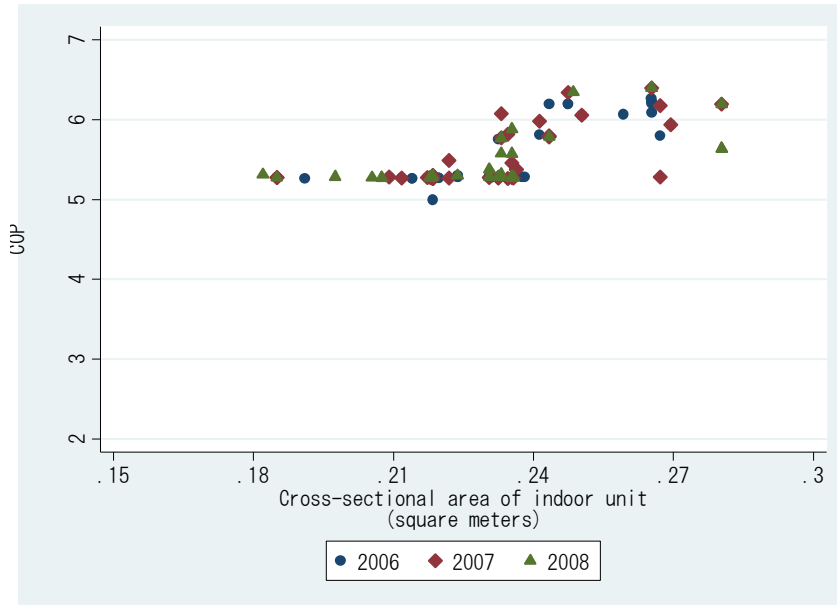
Figure 5. COP and Indoor Unit Size During 2006-2008
