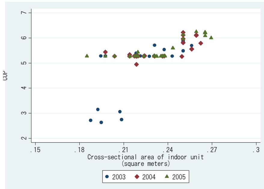
Figure 4. COP and Indoor Unit Size During 2003-2005
