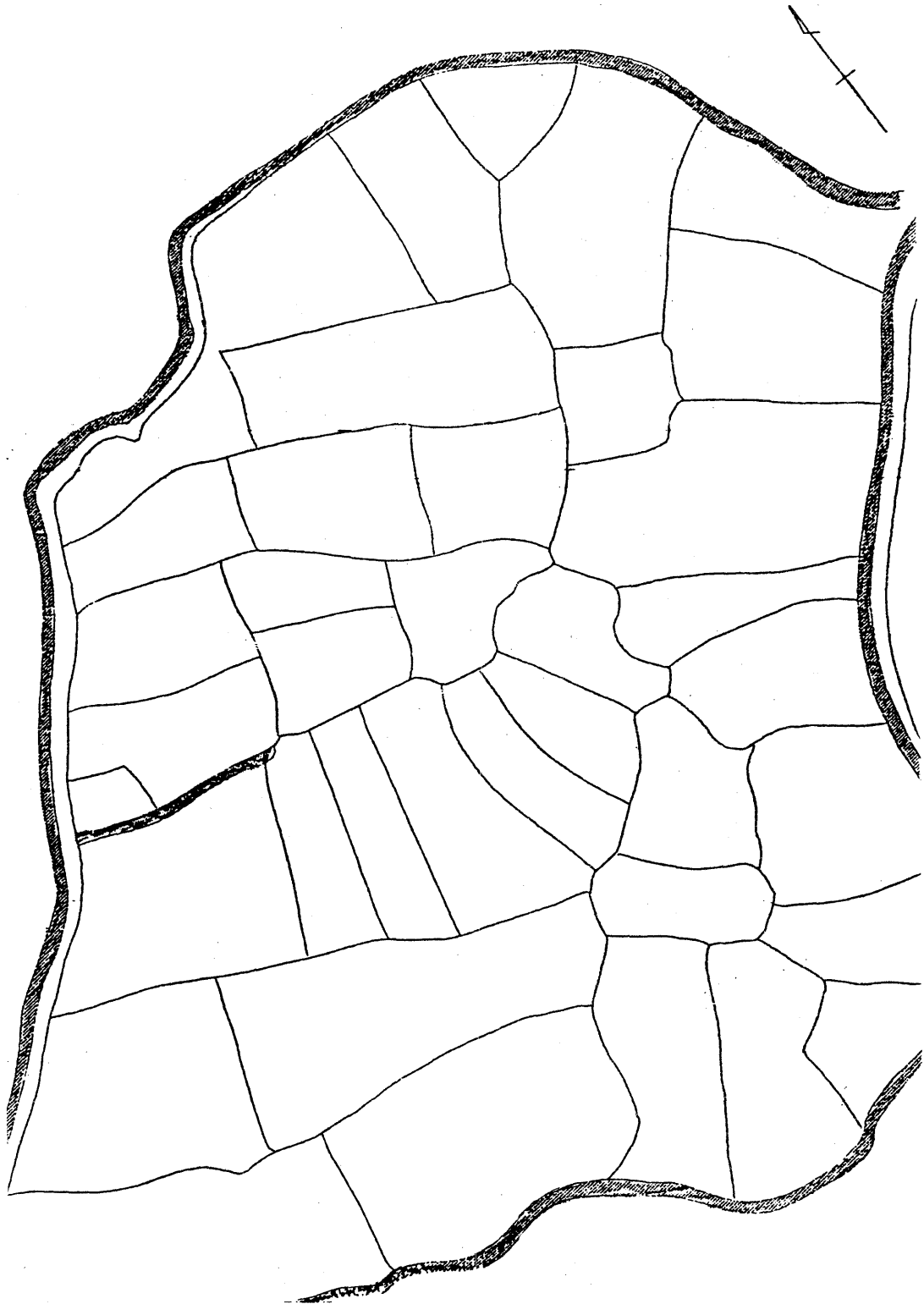
FIG. 4. Configuration of Paddy Fields Prior to Consolidation Project. Shaded lines are irrigation ditches.
